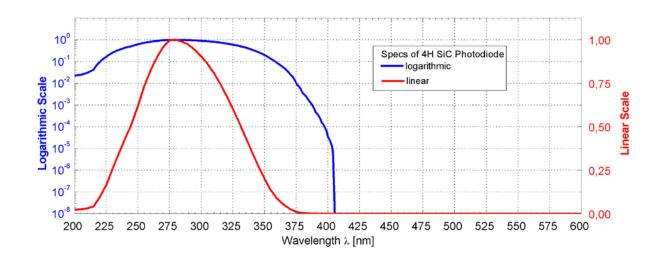
Broadband SiC based UV photodiode A = 1.82 mm<sup>2</sup>
